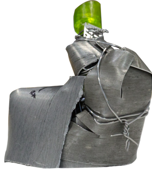
Figure 4.21: \text{NaCaNi}_2\text{F}_7 sample in sample holder with shielding in the form of boronated aluminium. The shielding is included in the simulations shown on figure 4.20.
