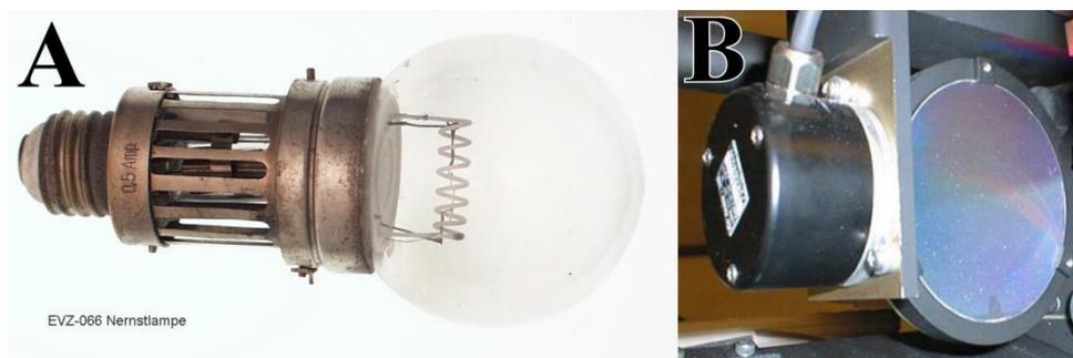
Figure 2-2. (A) The Nernst lamp with a ceramic rod by courtesy of Landesmuseum für Technik und Arbeit in Mannheim, Germany. (B) The halogen lamp with tungsten filament and halogen gas inside a glass capsule from a dispersive NIR spectrometer (6500, NIR systems, Inc.). Figure A is from [www.commonswikimedia.org](http://www.commonswikimedia.org).
