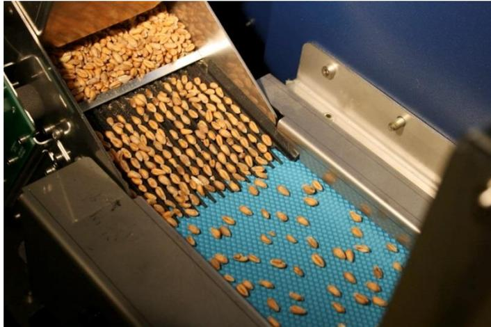
Figure 3-4. The EyeFoss from FOSS ([www.foss.dk](http://www.foss.dk)). Seeds are spread out on a conveyer belt to facilitate the image analysis on each single seed. Figure by courtesy of FOSS.
