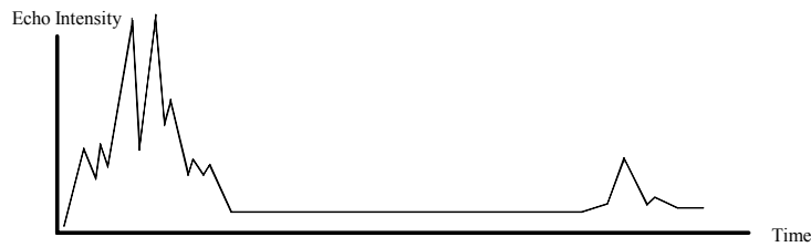
Figure 3. a) The pulse echo ultrasound principle is used. b) Double reflection may appear as false signals. c) Scatter occurs at reflections from small objects.
