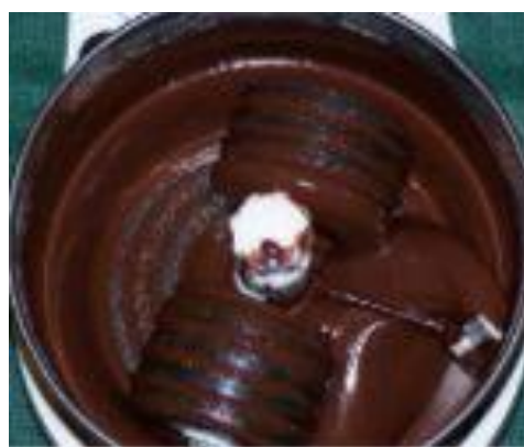
Fig. 10. Chocolate mixer (Melangeur) used for milling roasted cocoa beans to produce cocoa liquor.
