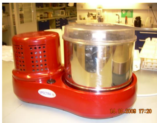
Fig. 10. Chocolate mixer (Melangeur) used for milling roasted cocoa beans to produce cocoa liquor.
