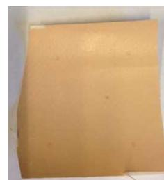
The membranes have three distinct layers; a membrane support layer that consists of polyester (PE), an active layer that is the filtering part of the membrane which consists of polyether sulfone (PES) for ultrafiltration membrane cartridges and polyvinylidene fluoride (PVDF) for microfiltration membrane cartridges, finally a residual fouling layer that consists of build-up (e.g. protein, minerals and fat) from the process (Figure 2.5).
