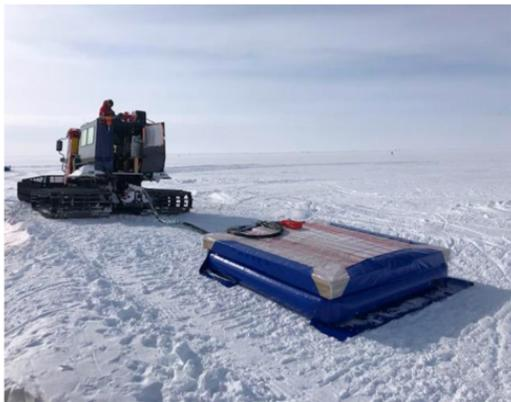
Fig. 3 The snow vehicle carries the UWB radar system was towing the dual-polarized antenna-array on the snow and taking measurements
