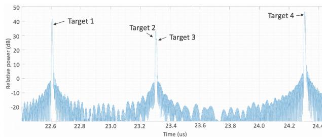
Fig. 5 Pulse compression simulation result of multiple point targets with different attenuations at different distance
