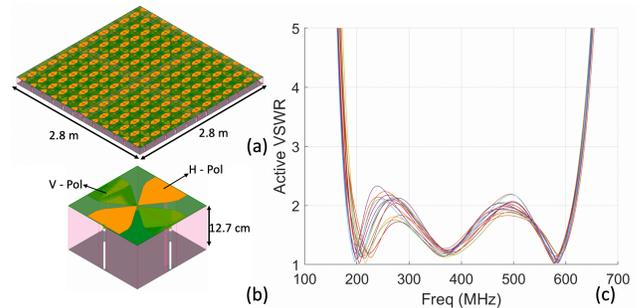
Fig. 2 UWB dual-polarized antenna array. (a) Structure of the full array (b) Structure of a single dual-polarized antenna element (c) Simulated Active VSWR of the full array
