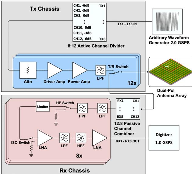
Fig. 1 Radar System Block Diagram
