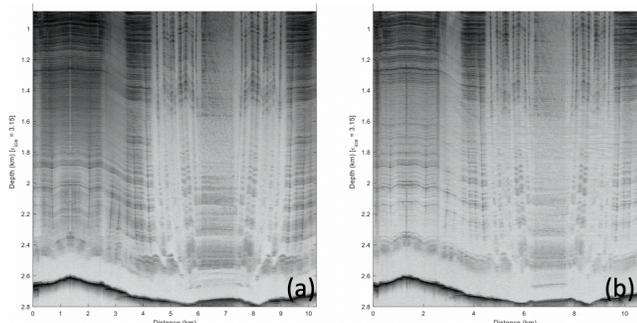
Fig. 4 Radar quick-look echograms of data collected in Northeast Greenland. (a) VV-Polarization (b) HH-Polarization
