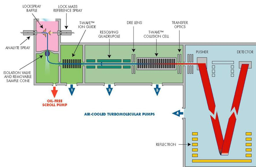
Figure 2. Schematic illustration of a Waters Q-TOF Premier mass spectrometer with a single V reflectron flight path. From Waters (2005) with permission.
