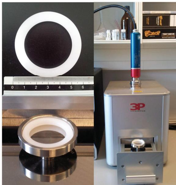
**Figure 1.** Intravaginal dapivirine ring. Experimental setup with the Raman pharmaceutical area testing (PhAT) probe placed on top of a ring spinner (3P innovation). Ring is placed in the small cup, which rotate when the drawer is closed.
