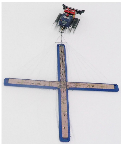
Fig. 12. Pistenbully tract vehicle towing Mills cross antenna array.
