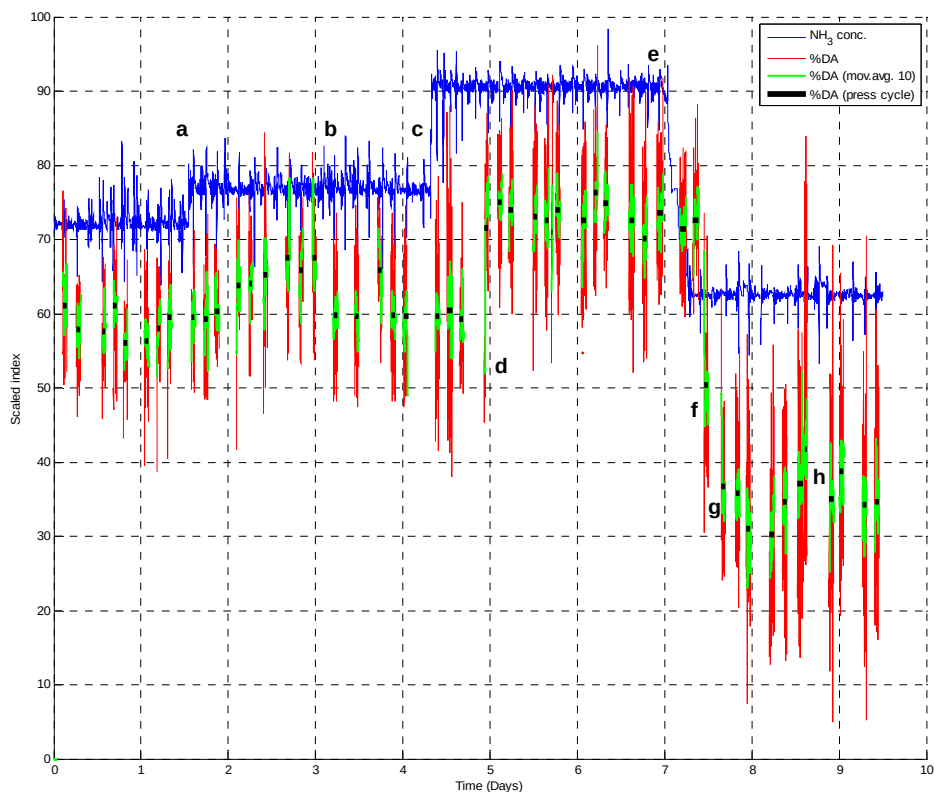
Figure 54 On-line ammonia prediction in the amidation reactors (blue) and in-line predicted %DA in pectin press cake (red, and moving average of 10 %DA observations is green, average of entire press cycle is black) in the screw press following the amidation. Both have scaled values on the y-axis. See the text for further details.
