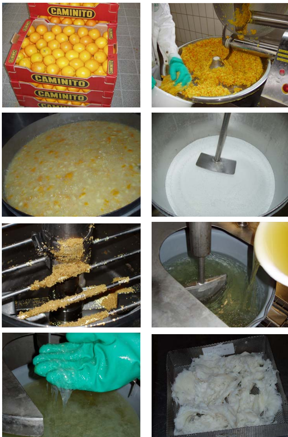
Figure 42 Various processing stages of pectin in pilot plant scale. From top left to bottom right: Raw material (oranges), chopped peel, extraction, filtration (filter aid), ion exchange (resin), precipitation, precipitated pectin and wet pectin press cake.
