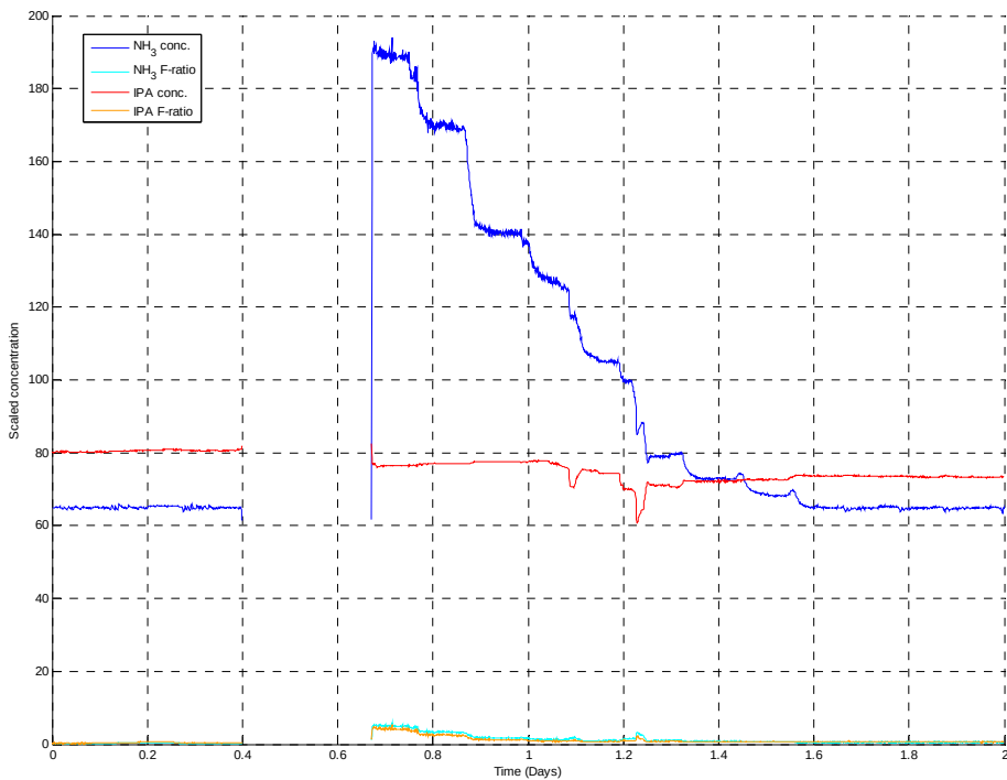
Figure 56 Scaled ammonia concentration before and after a 6½ hour power failure affecting the factory.
